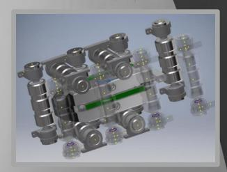
The module is installed on dummy bar using a custom designed adapted and execute the measurement cycle during the bottom-to-top or top-to-bottom dummy bar movimentation.
